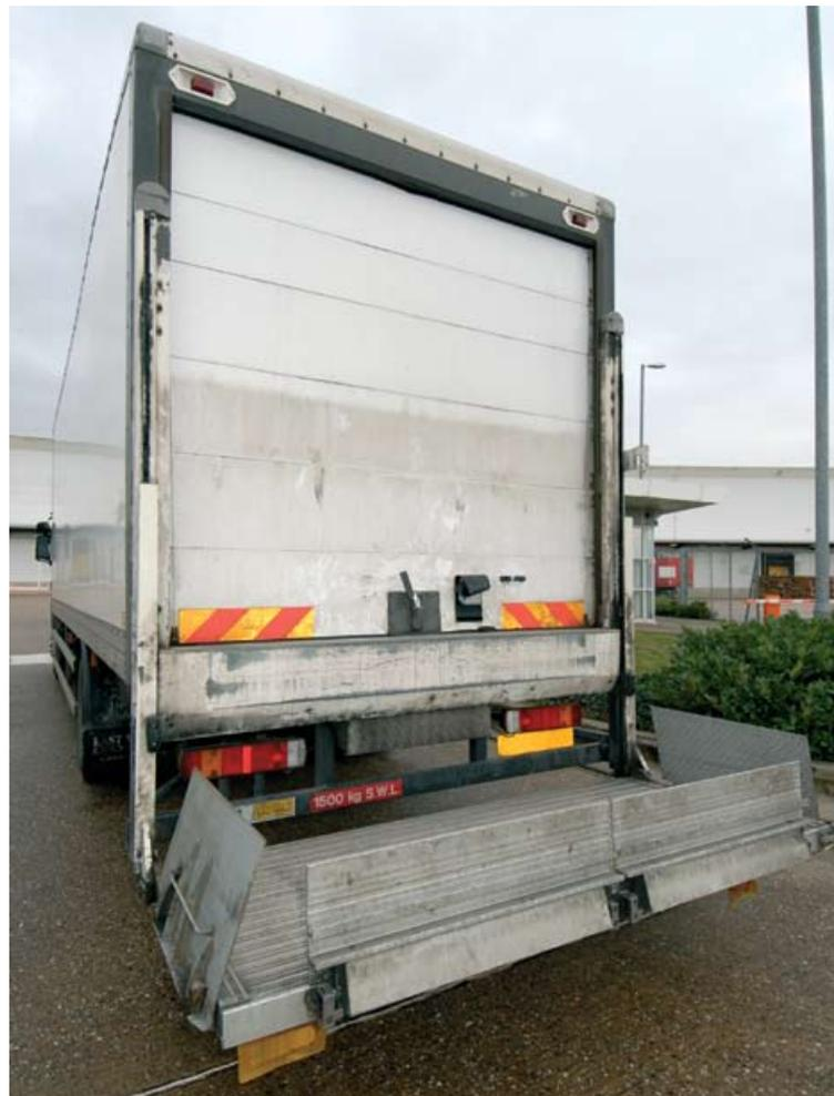
**Figure 31** Vehicle with tail lift
