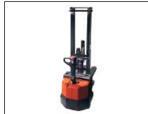
**Figure 3** Pedestrian operated pallet stacker
