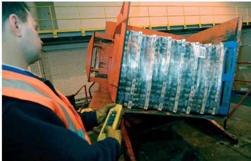
**Figure 45** Pallet inverter
