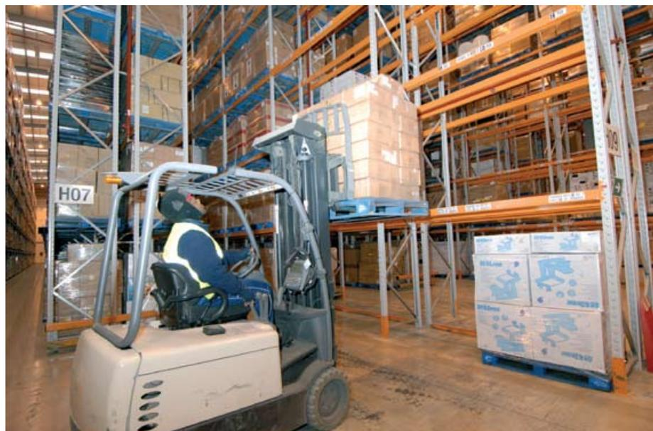
**Figure 18** Counterbalanced fork-lift truck
