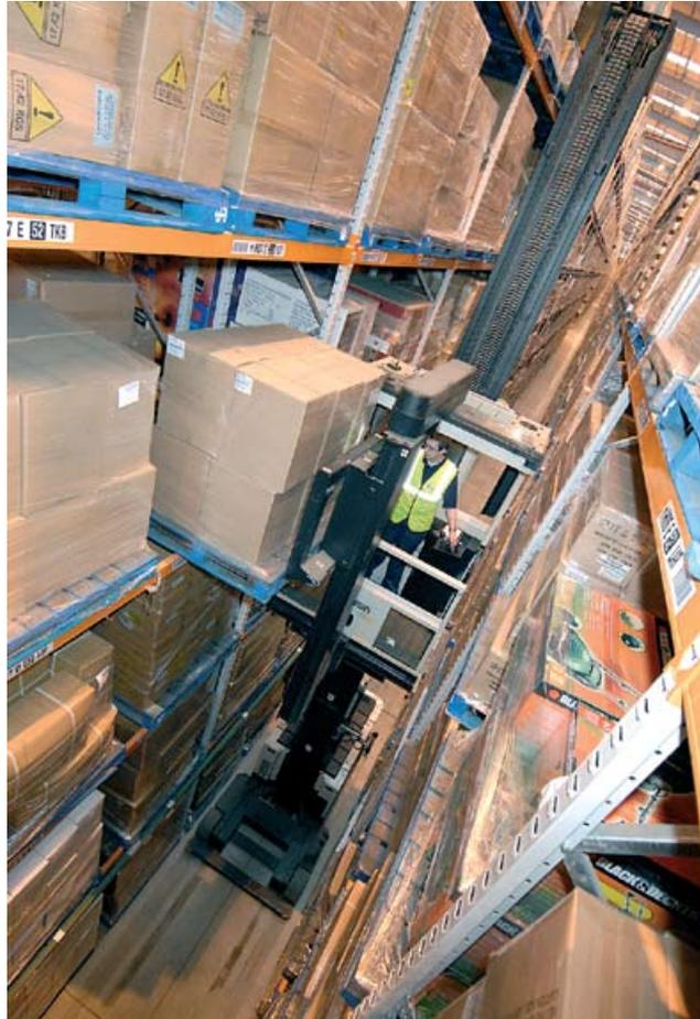
**Figure 21** Very narrow aisle man-up truck
