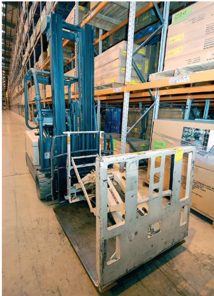
**Figure 19** A fork-lift truck with push-pull attachment
