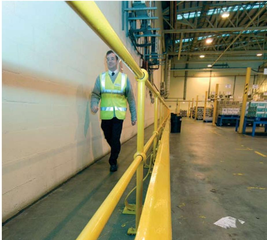
**Figure 26** Pedestrian/vehicle segregation
