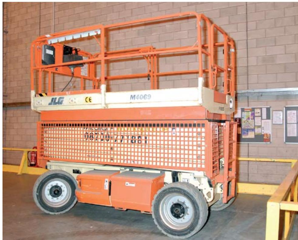
**Figure 34** Mobile elevating working platform (MEWP)
