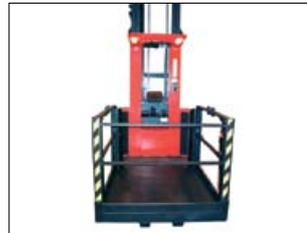
**Figure 2** High-lift platform truck
