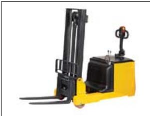
**Figure 1** Pedestrian operated counterbalanced fork-lift truck
