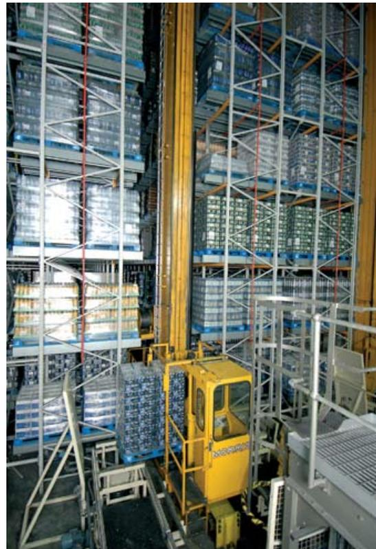
Figure 54 Rail-dependent storage and retrieval machine with operator cabin
