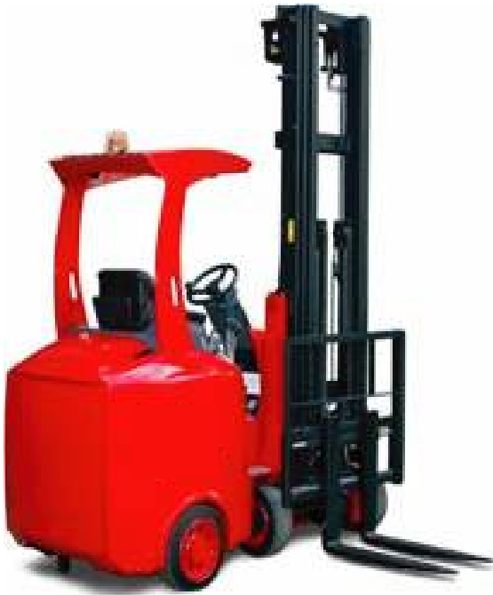
Articulated narrow aisle truck (type 2)
