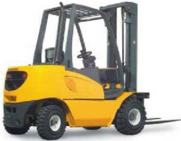
4 Wheel counterbalance truck (type 1)
